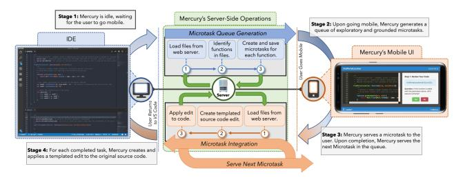
Figure 5: Mercury's architecture supports four stages of interaction.
